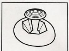
To reset the neutral position once the game has started, let go of the Control Stick so it can return to its center position (as shown in the picture on the left) then press START while holding the L and R Buttons.
